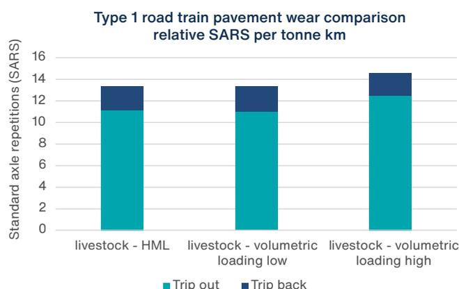
**Figure 3. Pavement wear comparison for livestock heavy vehicles only – per tonne-km payload.**
