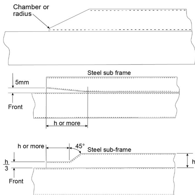
Figure 18: Examples of progressive load bearing transition
