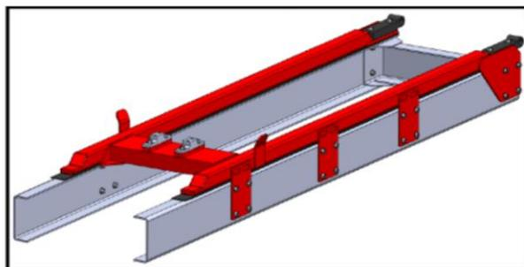
Figure 28 - Tipper sub-frame with integrated load cells
