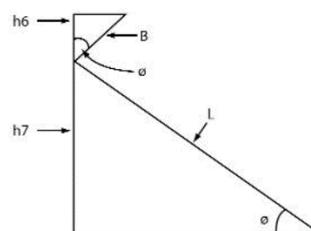
Figure 31 – Height of centre of gravity
