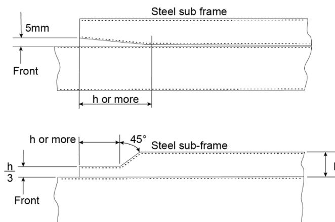
Figure 2: Examples of progressive load bearing transition
