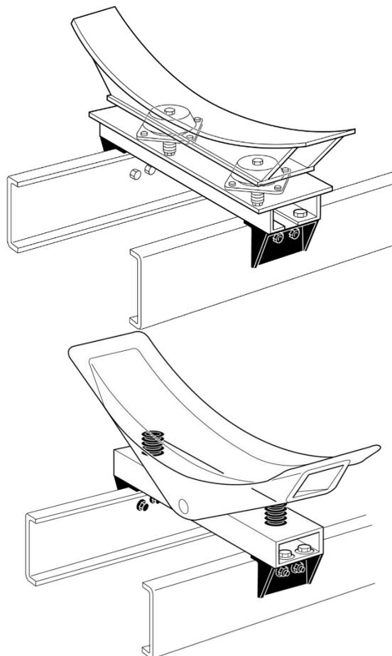
Figure 9: Details of a typical front mounting bracket
