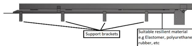
Figure 23 – Example of Support Bracket configuration
