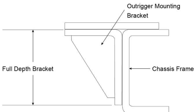
Figure 11: Details of a typical chassis mounting bracket
