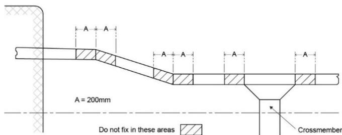
Figure 4: Attachment locations chassis
