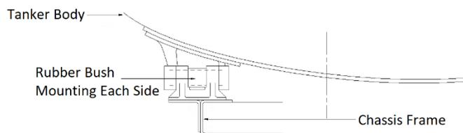
Figure 10: Details of a typical rear mounting bracket
