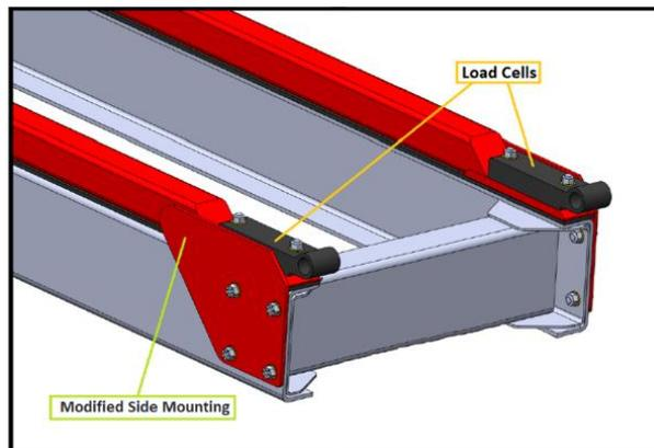
Figure 27 - Example of load cells mounted to modified sub frame that maintains structural integrity. In this example, by enlarged and thickened mounting plates with upside down countersunk fasteners to prevent bolting through chassis flange)
