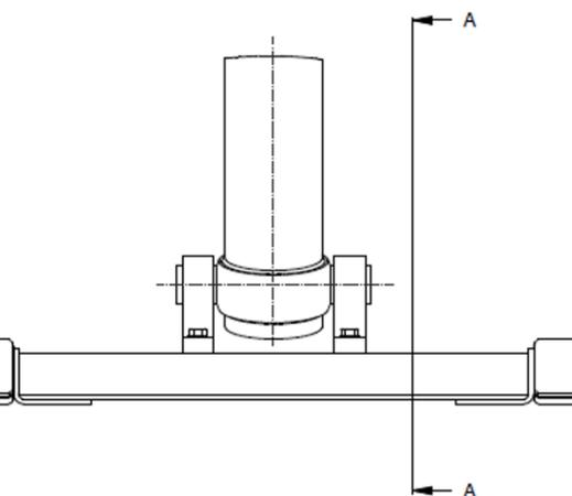
Figure 25 - Typical installation of the hoist cylinder.
