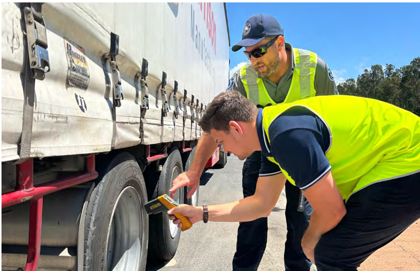
SCO Scott and Customer Experience and Engagement Officer, Carlo checking brake temperatures at Chinderah HVSS.
