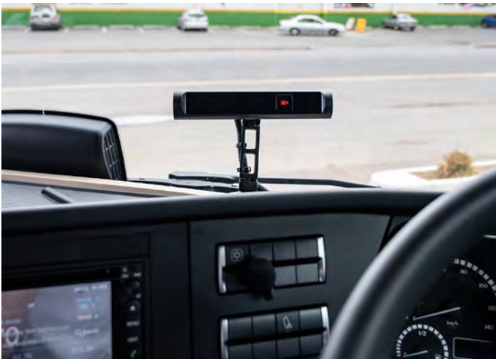
Fatigue and Distraction Detection Technology delivers immediate alerts to drivers when it senses potential fatigue or distraction.
