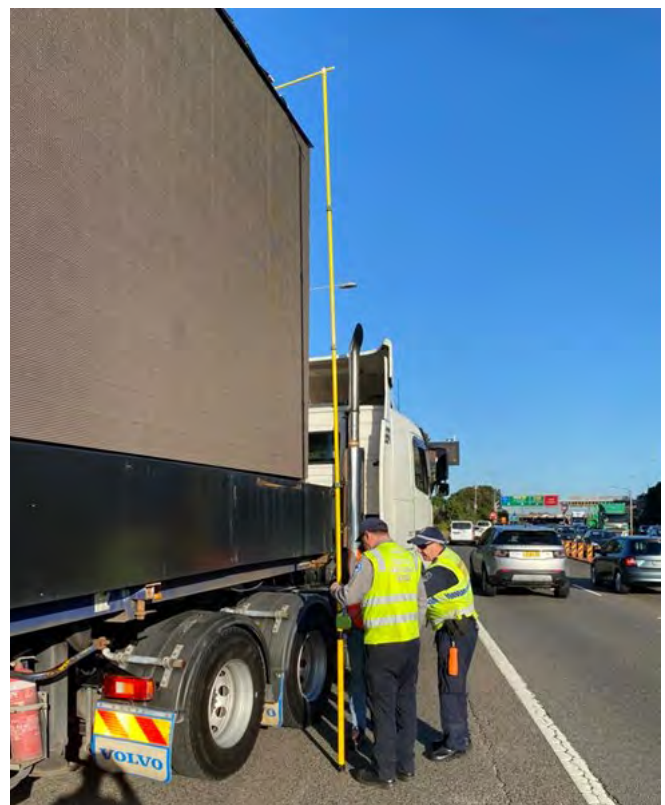
SCOs inspecting an over-height vehicle after it activated the vehicle height detection warning system in Sydney.
