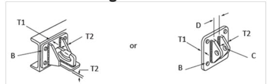
Figure 3.6 Typical attachment of chains
