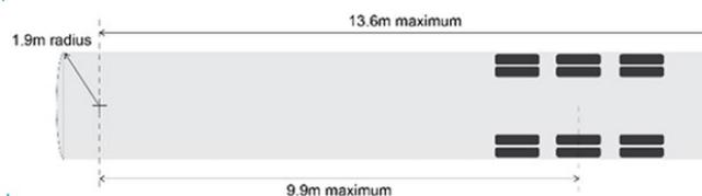
Figure 16.1 Semitrailer
