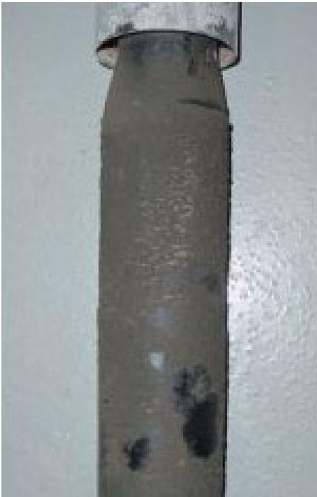
Figure 4.4 Examples of misting shock absorbers
