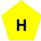
Number plate label for vehicles fuelled with hydrogen:
