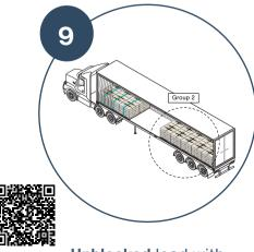
**Unblocked** load with rated curtains
