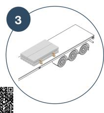
Tie-down restraint with chains – Precast concrete panels on a flat tray
