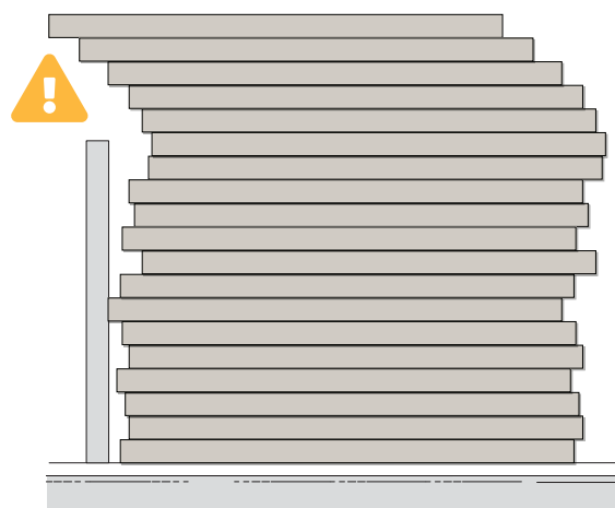
Figure 371 Unblocked top portion of load
