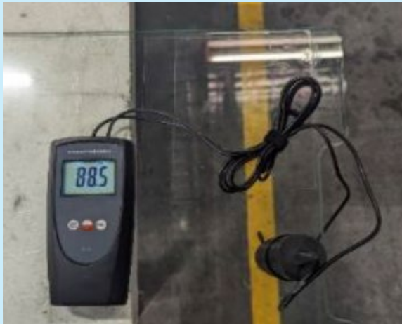
Figure 8: An example of glazing with anti-shatter/ glare film being tested for VLT.
