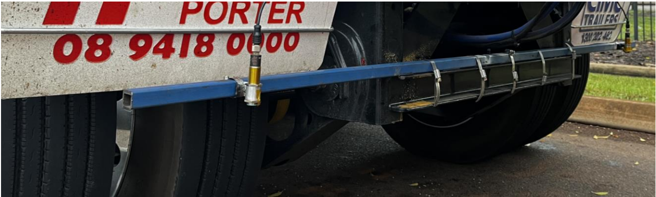
Figure 6 - Ultrasonic distance measurement sensors recording wheel path vertical profile
