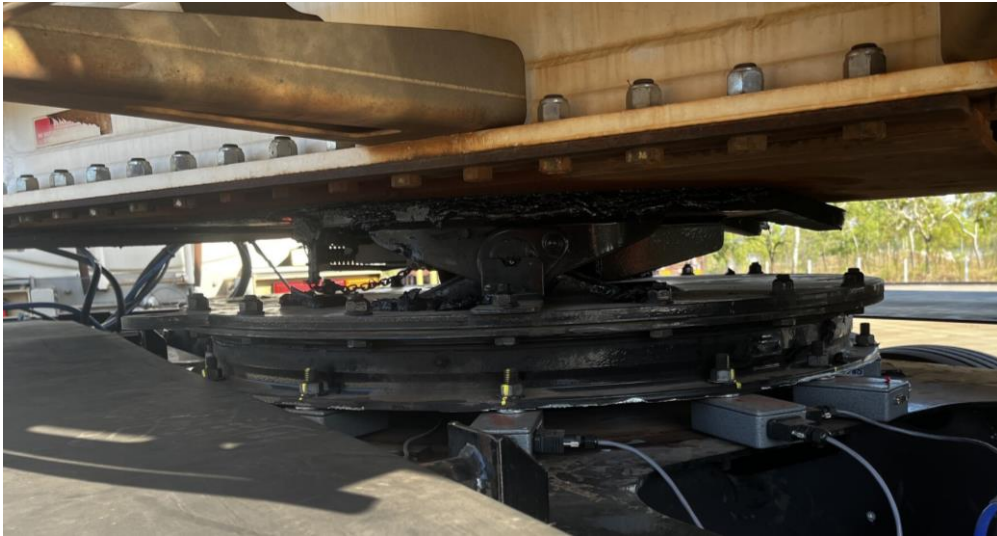
Figure 13 - Test Dolly fifth wheel oriented at 54° away from proper position during first (rear dolly) test
