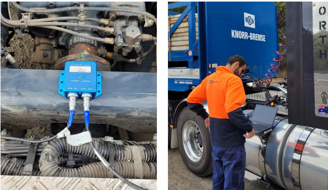
Figure 3.3: Vehicle sensor (IMU) positioned on prime mover cross member
