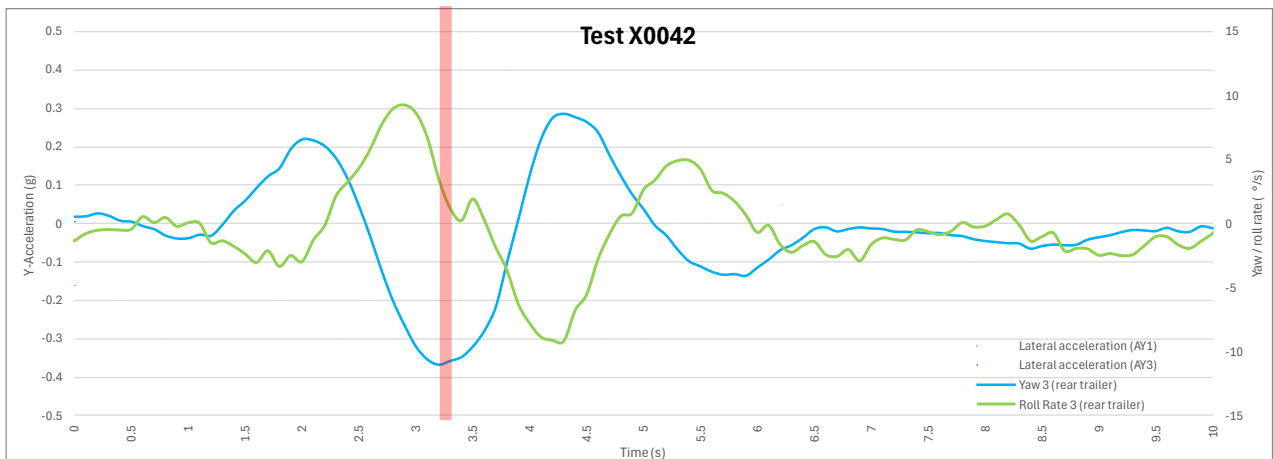
Figure A.16: Test X0042 – roll and yaw rate (EBS all OFF)
