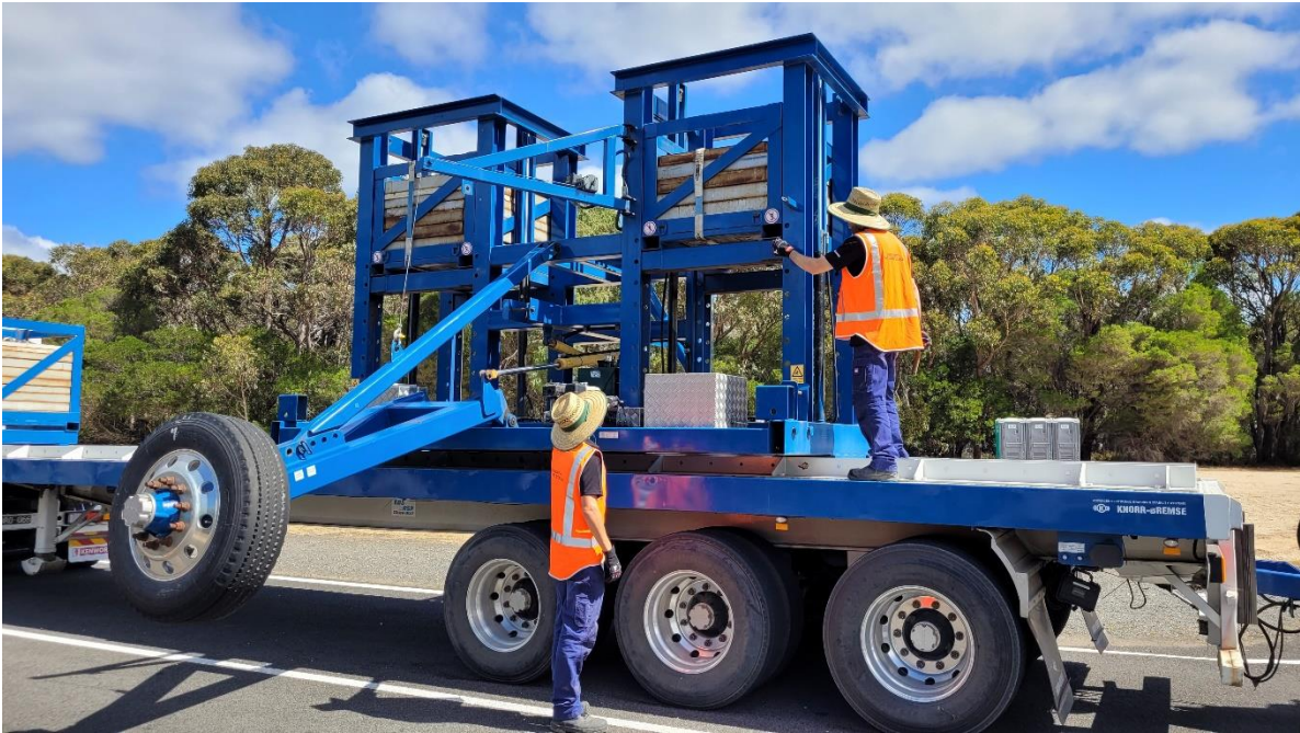
Figure 3.5: CoG height of the lead trailer being adjusted during testing
