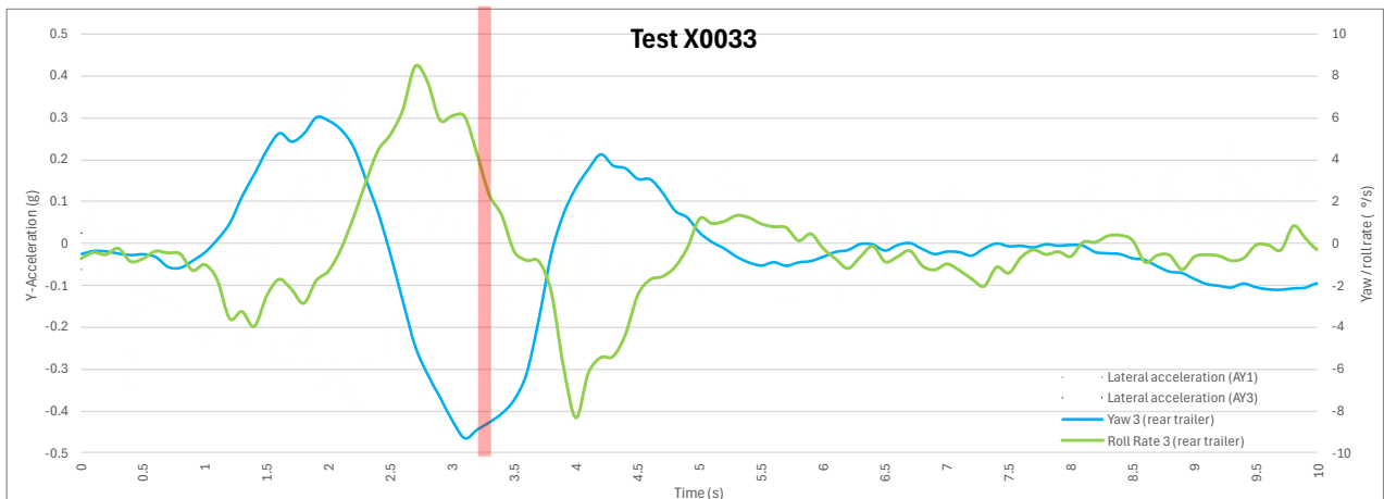
Figure A.10: Test X0033 – roll and yaw rate (EBS ON/OFF/ON)
