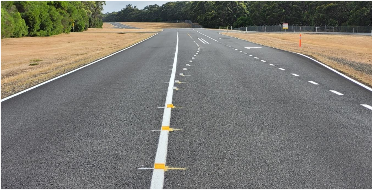
Figure 3.4: Lane change path as marked for testing on AARC highway circuit
