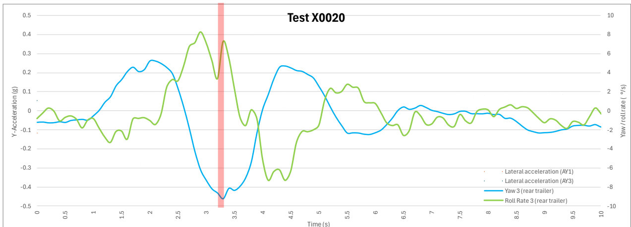
Figure A.4: Data trace for test X0020 – yaw and roll rate (EBS all ON)
