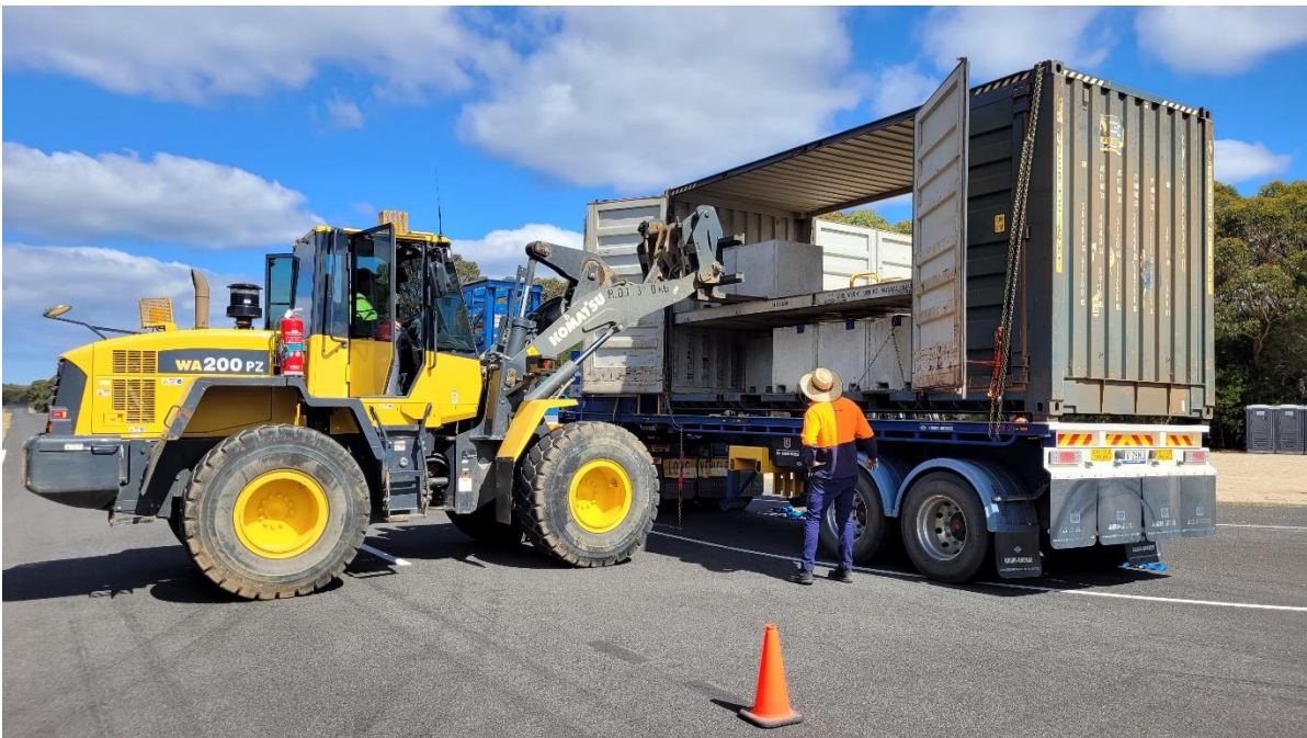
Figure 3.6: CoG height of the rear trailer being adjusted during testing
