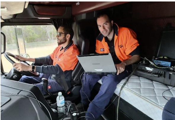
Figure 3.1: Field engineers fitting sensors and configuring data acquisition system
