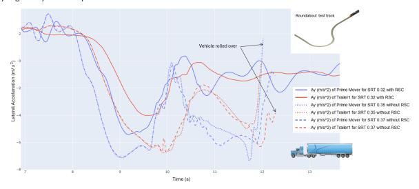
Figure 21 Lateral acceleration of prime mover semitrailer at roundabout test track showing effectiveness of RSC
