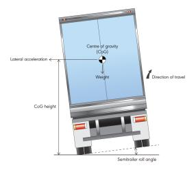
Figure 1 Static Rollover Threshold illustration
