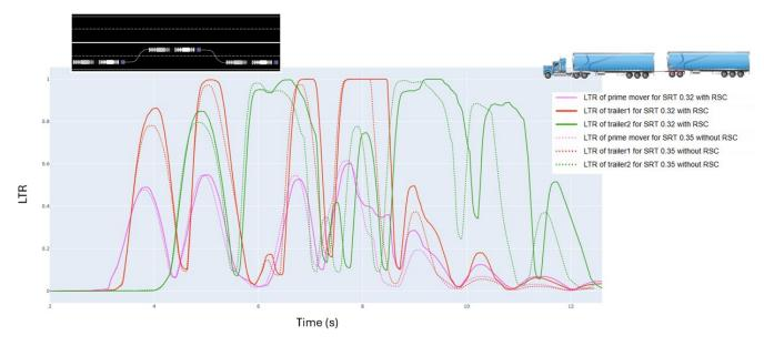
Figure 37 Double Lane Change test of A-Double showing effectiveness of RSC in LTR
