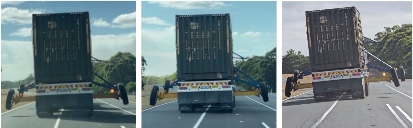
Figure 11 2024 Anglesea testing RSC All ON vs Dolly OFF vs All OFF RA comparison
