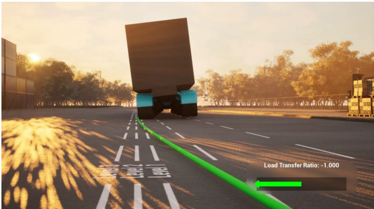
Figure 6 A compliant L2 PBS Truck and Dog passing HSTO with an LTR of 1 (w. right side wheels in the air)
