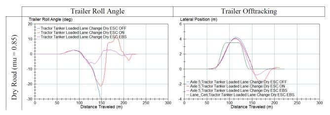
Figure 10 Plots of lane change for a loaded vehicle - roll and tracking errors. (UMTRI U31 Figure 3-48)
