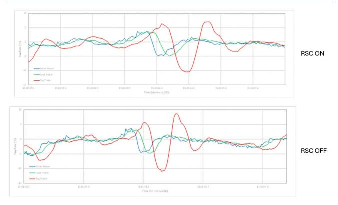
Figure 13 Yaw rates recorded for each vehicle unit from field testing by NTRO.
