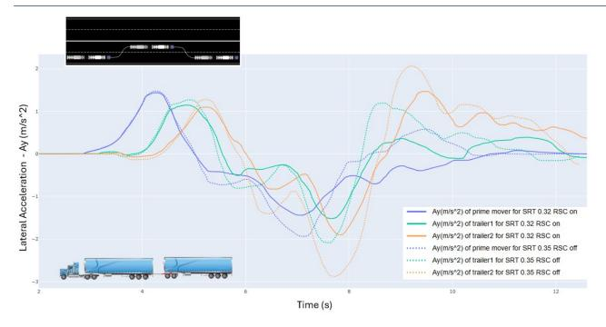
Figure 36 Double Lane Change test of A-Double showing effectiveness of RSC in lateral accelerations
