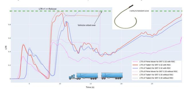
Figure 28 LTR of A-double at J-entry to transient curve test track showing effectiveness of RSC
