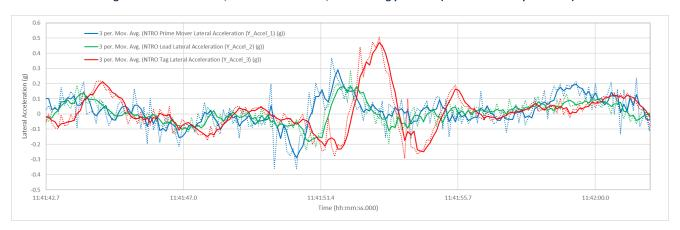
Figure 18 Prime mover, lead trailer, and rear trailer lateral acceleration comparison (Germanchev unpublished)
