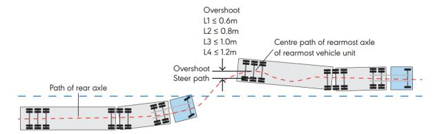
Figure 4 High-Speed Transient Offtracking illustration
