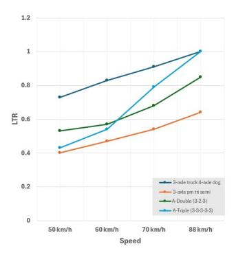
Figure 42 Impact of test speed on LTR
