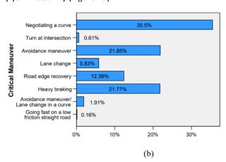
Figure 19 (a) Critical manoeuvre for trucks with loss of control (b) Critical manoeuvre for trucks with only yaw instability (Kharrazi and Thomson 2008)
