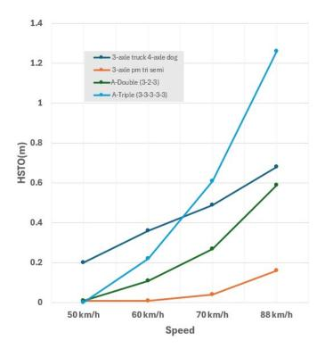
Figure 41 Impact of test speed on HSTO
