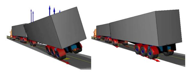
Figure 29 An A-double undertaking a lane change manoeuvre - where both trailers are equipped with RSC on the left, but not on the dolly, versus the trailer and the dolly all fitted with RSC on the right
