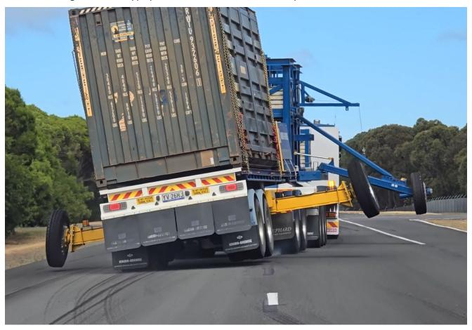
Figure 15 Activation of the RSC on the dolly providing additional stability control under an emergency evasive manoeuvre
