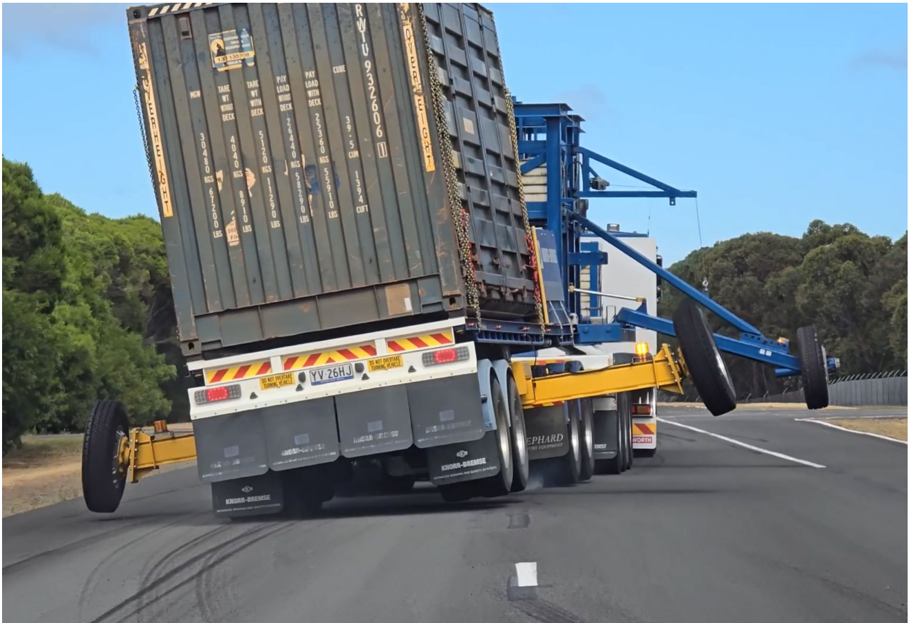
Figure 15 Activation of the RSC on the dolly providing additional stability control under an emergency evasive manoeuvre
