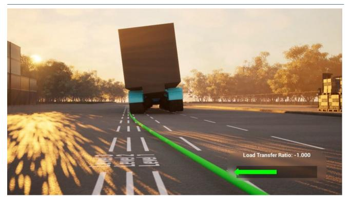
Figure 6 A compliant L2 PBS Truck and Dog passing HSTO with an LTR of 1 (w. right side wheels in the air)
