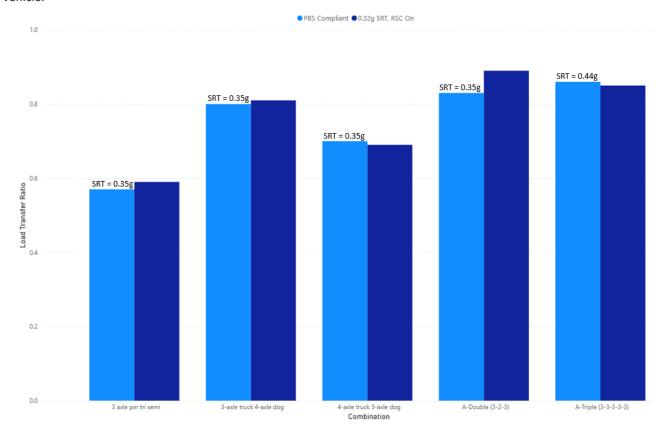
Figure 34 Load Transfer Ratio of Lane Change vehicles
