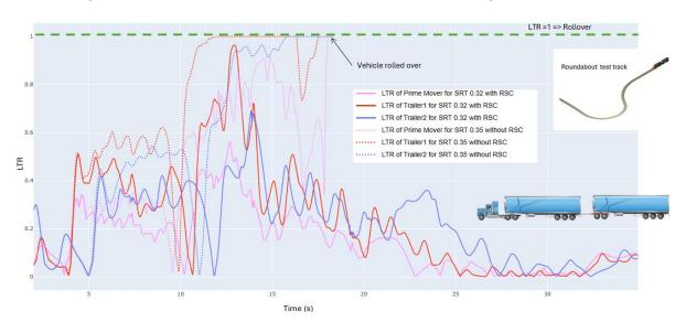
Figure 24 LTR of A-double at roundabout test track showing effectiveness of RSC
