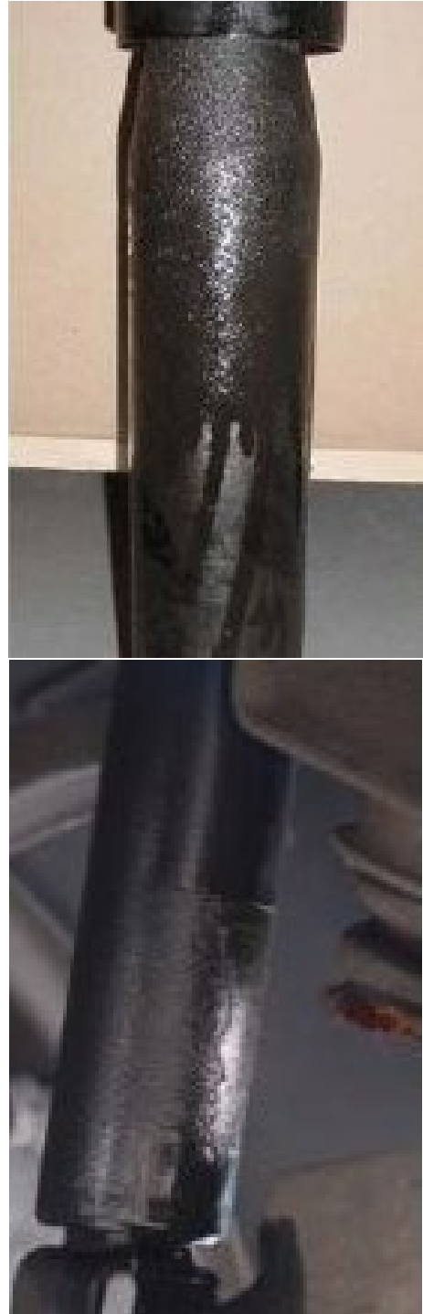
Figure 4.5 Examples of leaking shock absorbers
