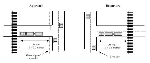
Figure 2. Stacking distances at railway level crossings (Main Roads WA 2003)
