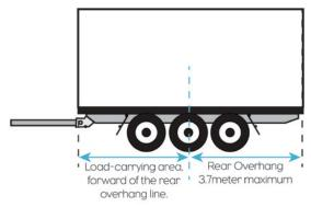
Rear overhang on a pig trailer must not exceed the lesser of the length of the load-carrying area, forward of the rear overhang line or 3.7 metres.
