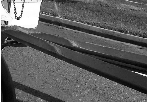
Figure 18: Wear on drawbar
