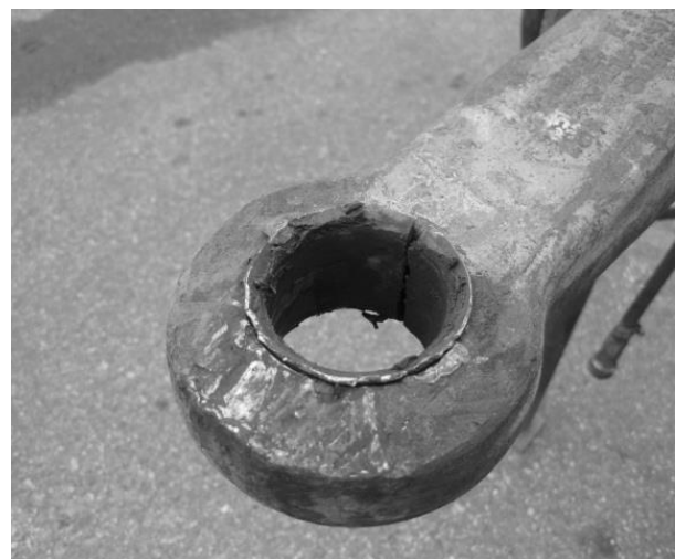
Figure 11: Heavily worn and damaged drawbar eye bush
