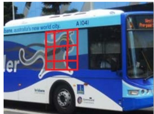
Courtesy of Dave Brown via Flickr Figure 4: Breakable side exit Red lines indicate where film should be cut or a gap left
