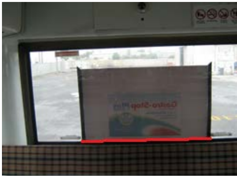
Figure 1: Push-out emergency exit (inside) Red line indicates where film should be cut or a gap left
