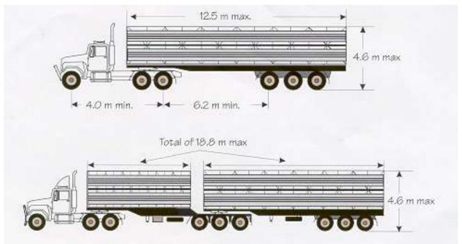
B-Doubles must comply with the axle spacings as specified in Part 2 of the *Vehicle and Traffic (Vehicle Operations) Notice*, relating to B-Doubles.
