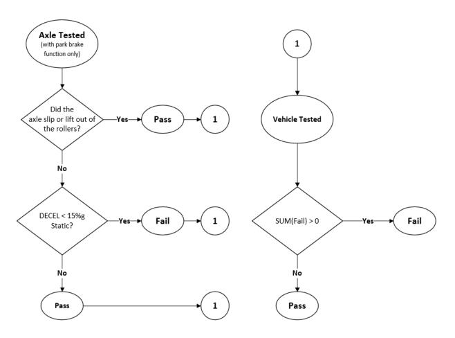
Emergency and park brakes that act on the wheel ends are assessed at the axle level. If all axles that deliver an emergency and/or park brake functionally pass the above test, the vehicle passes the test.
