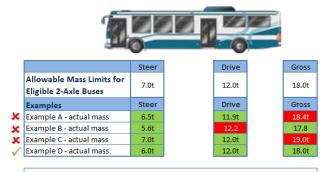
Example A - The steer and drive axle mass are within allowable limits, however the vehicles Gross Mass has exceed the 18.0t allowable limit by 0.4 tonne
