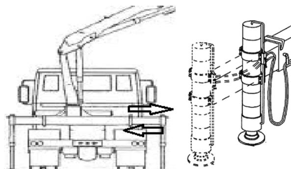
Figure 1: Examples of stabilisers/outriggers
