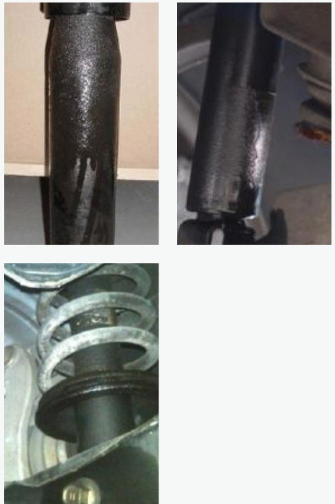
**Note:** Some minor streaking of oil may appear on a new shock body during initial stroking. This is the result of the seal 'setting' and purging any oil (from assembly) from the seal. This is not to be mistaken as a failure, as it is temporary and totals only a few millilitres of oil.
