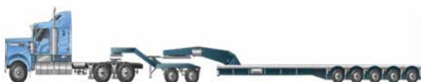
Figure 3 Example of a prime mover, low loader dolly and 5 axle low loader
