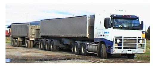
A Medium Articulated Vehicle towing a Dog Trailer (commonly known as a MAD) and a Medium Articulated Vehicle towing a Pig Trailer (MAP) meet the definition of road train under the Heavy Vehicle National Law (HVNL) and is a Type 1 road train as its overall length is less than 36.5m.
