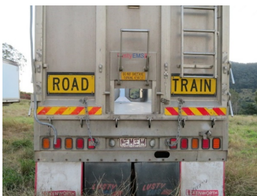
Figure 1: Road train trailers do not require a coupling fitted to the rear of the unit.
