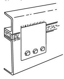
Figure 7: Typical fish plate attachment
