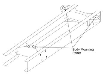
Figure 12: Typical three-point mounting
