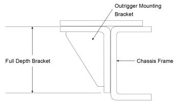
Figure 11: Details of a typical chassis mounting bracket
