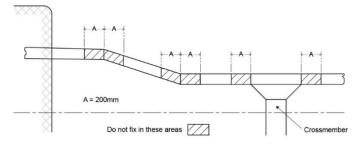
Figure 4: Attachment locations chassis
