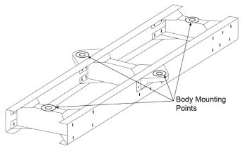
Figure 13: Typical four-point mounting
