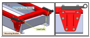
Figure 26 -Option 1 Example: Load cells w/ integrated pivot mounted on brackets & integrated into sub-frame
