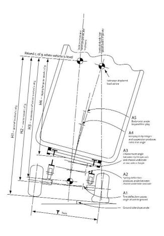
Figure 30 – Values to determine tipper stability
