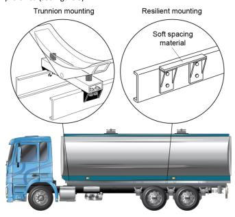
Figure 8: Typical example of tanker mounting
