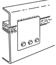
Figure 20: Typical fish plate attachment
