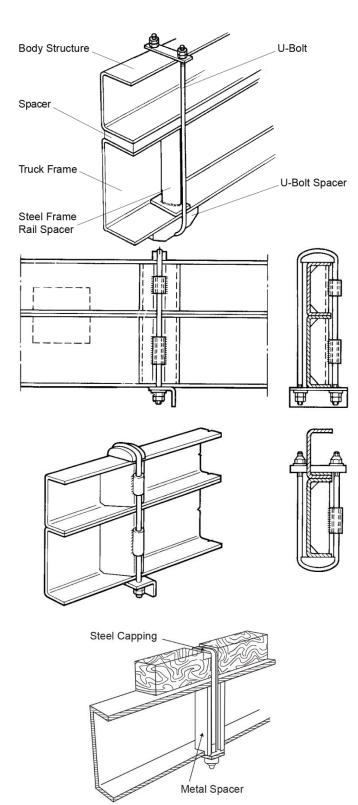
Figure 5: Typical U-bolt body mountings
