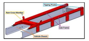
Figure 21- Basic Tipper Sub-Frame
