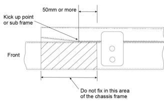
Figure 3: Attachment front end of sub-frame
