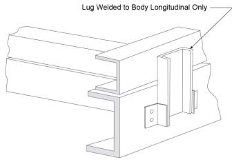
Figure 15: Additional horizontal restraint used with some body mountings
