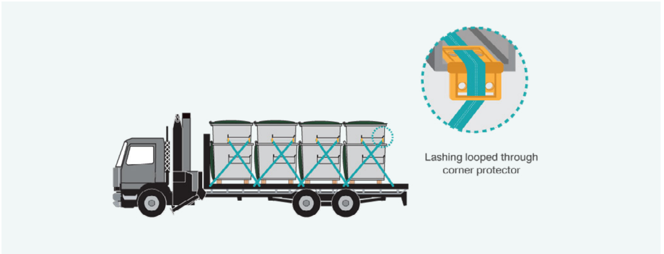
Figure 9. Double stacked empty bins. Lashing with corner protector.
