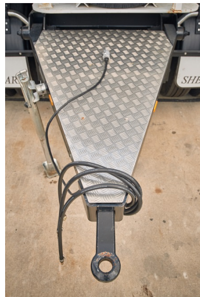
Figure 2: Dog trailer correctly fitted with rubber hoses
